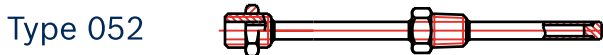
Type 052 11 mm OD or 1/4" NB, Parallel or Tapered Thread 1/2" BSP(PI) Running Nipple
